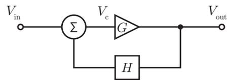
Transmission du circuit :  $\frac{V_{out}}{V_{in}} = \frac{G}{1 - H G}$
