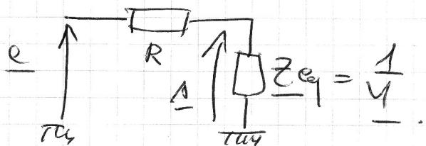
$$\underline{H}' = \frac{\underline{1}}{\underline{e}} = \frac{\underline{Z}_{eq}}{R + \underline{Z}_{eq}} = \frac{1/Y}{R + 1/Y} = \frac{1}{1 + RY}$$
